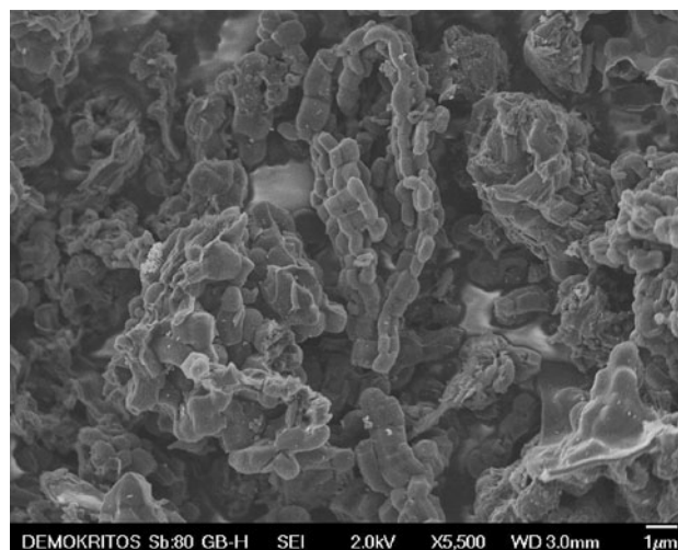
Fig. 1 SEM image of the doped \text{C3Pd} material (scale: 1 \mu\text{m} )
